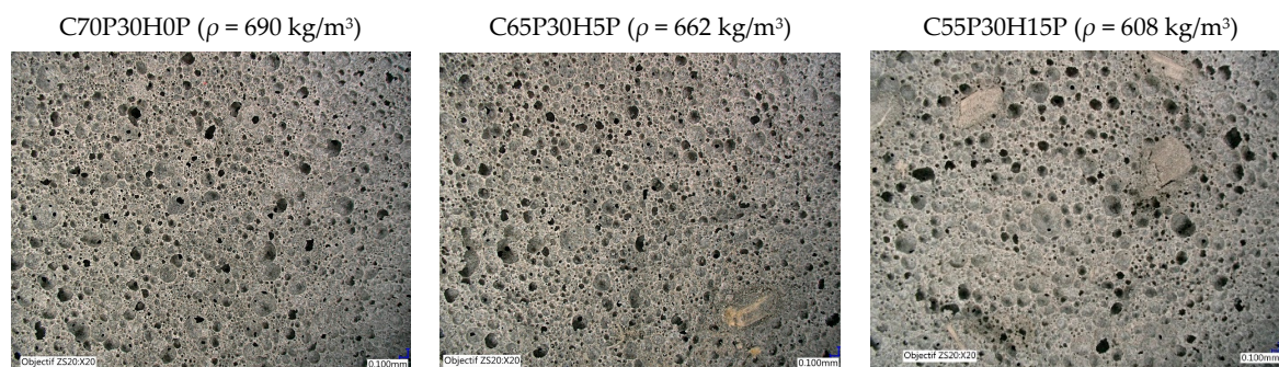
Figure 11. Microscopy images of porous structure evolution with increasing amount of hemp shiv using the preformed method.
